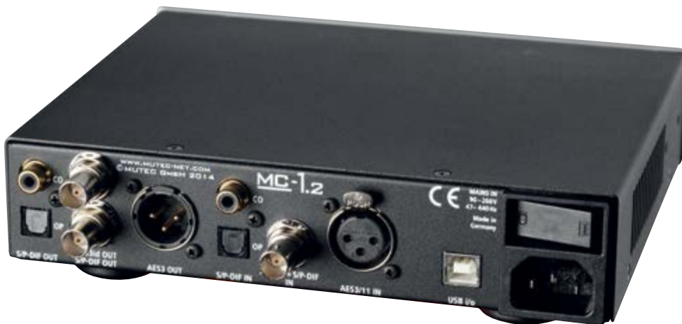
The USB data stream can be transferred to the formats AES3id, AES3 or S/P-DIF to a digital-to-analog converter.
